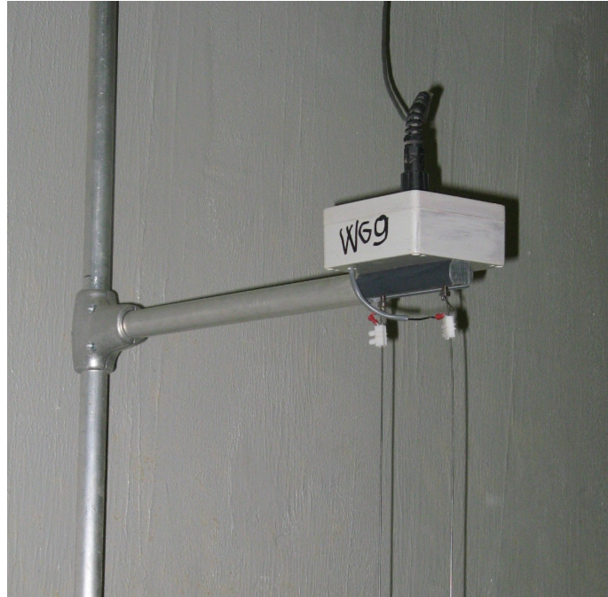
Figure 6. Resistive wave gauge.
